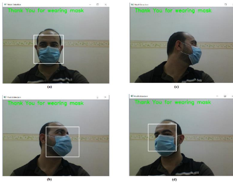
Figure 7. Effect of angle on detection (a) 0^\circ , (b) 45^\circ , (c) 90^\circ , and (d) -45^\circ .
