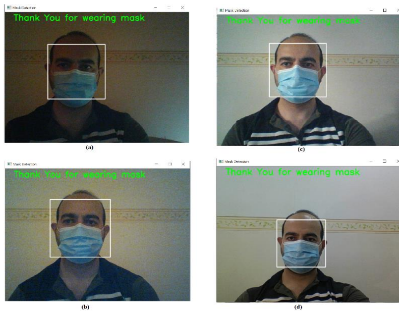
Figure 6. Effect of light on detection (a)10 lux, (b) 30 lux, (c) 90 lux, and (d) 140 lux.
