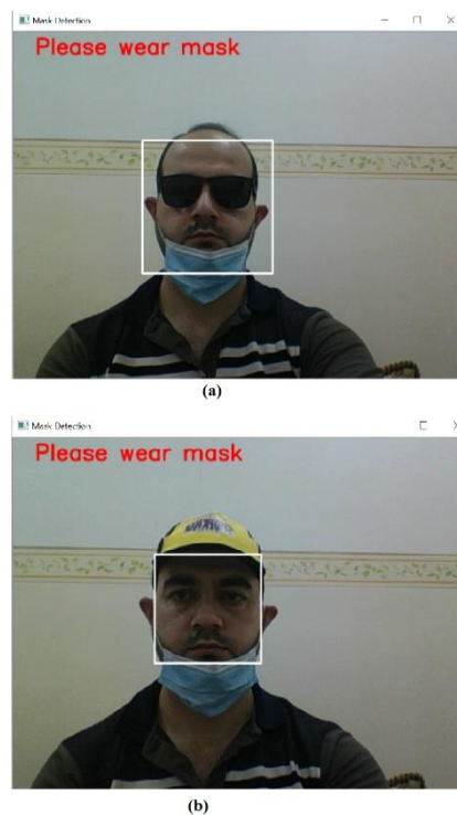
Figure 9. Effect of different face accessories (a) Sunglasses, and (b) hat cap.
