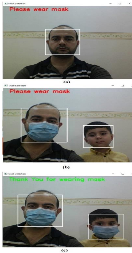
Figure 5. Face and mask detection (a) one person, (b) two persons not wearing one of the other, and (c) both wears.
